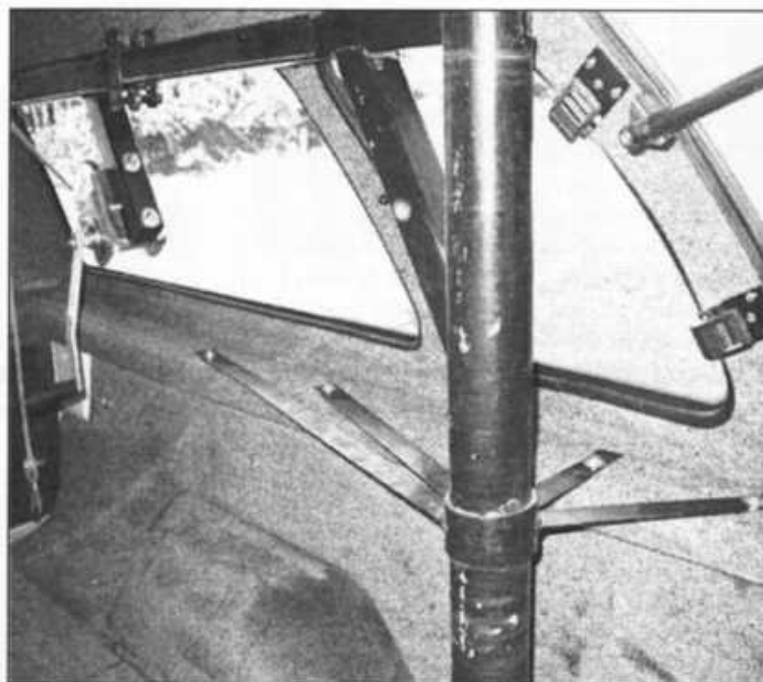
Lateral bracket mounts to bed sidewall and evenly distributes lifting force in all boom positions.
