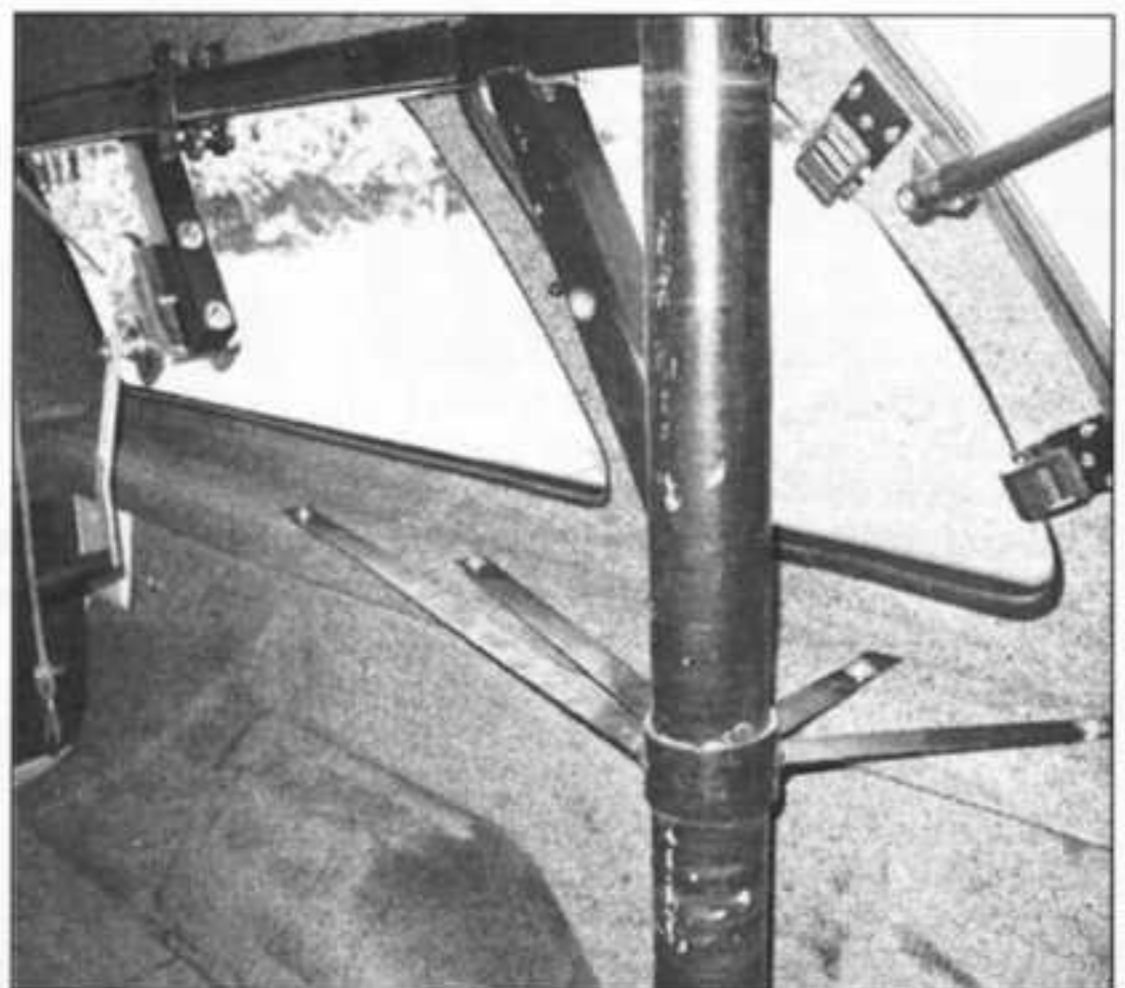
Lateral bracket mounts to bed sidewall and evenly distributes lifting force in all boom positions.
