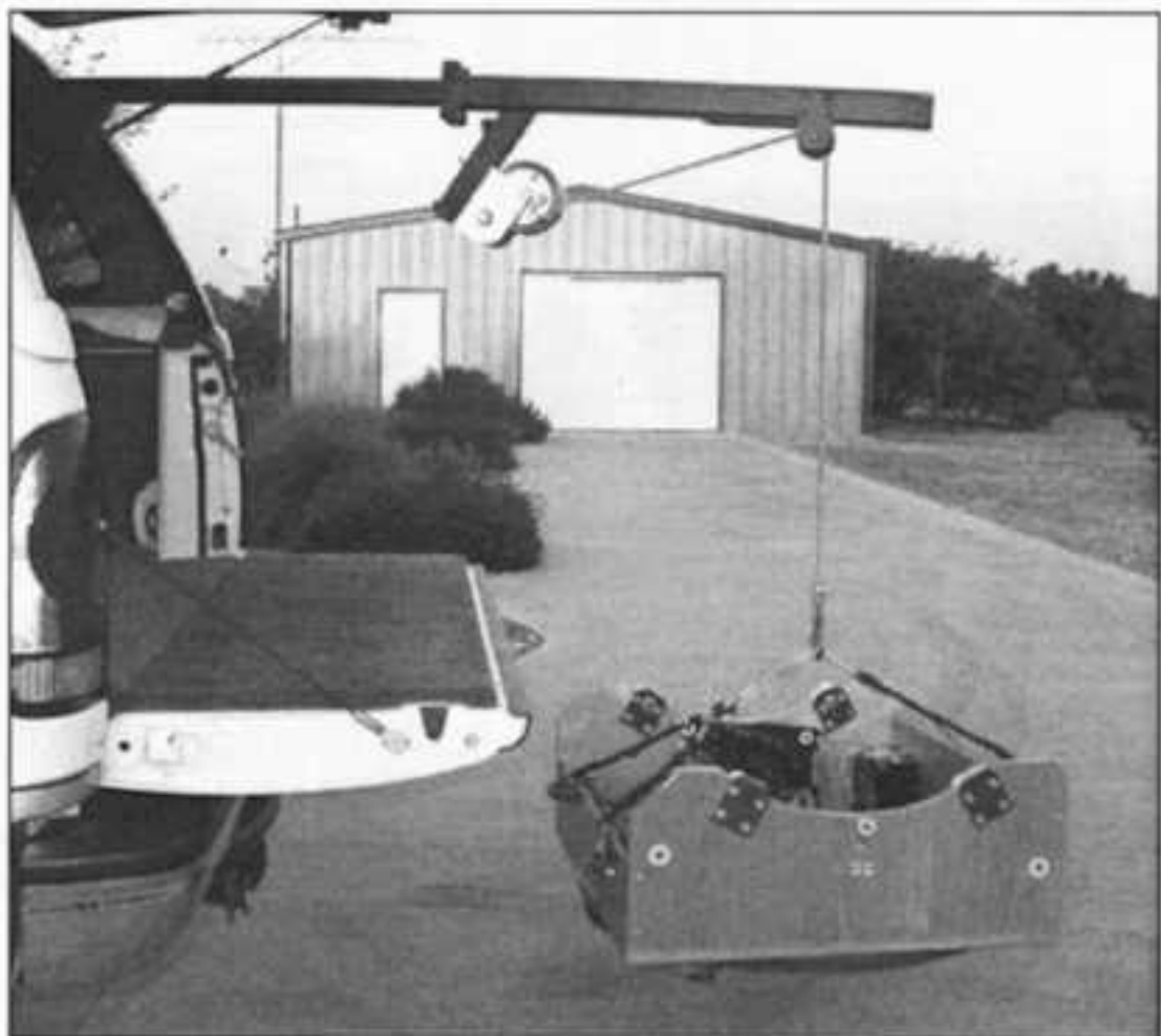
Engine hoist with extended boom provides easy lifting of telescope components from well inside truck bed.
