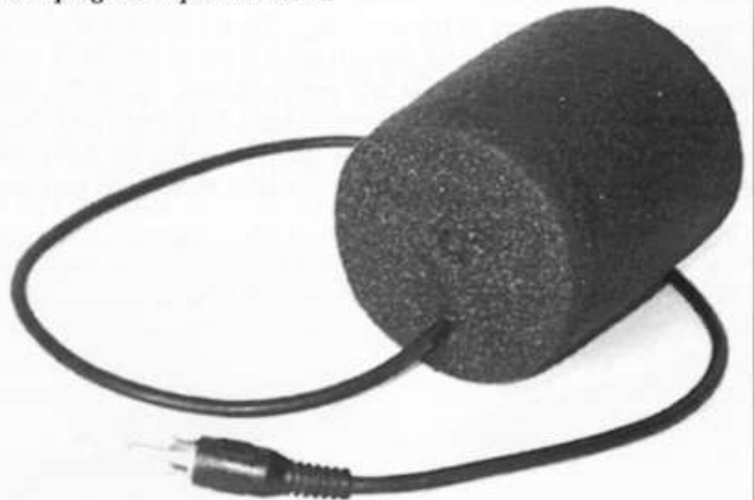
Heat is generated by several ceramic resistors placed in series and powered by 12 VDC.
