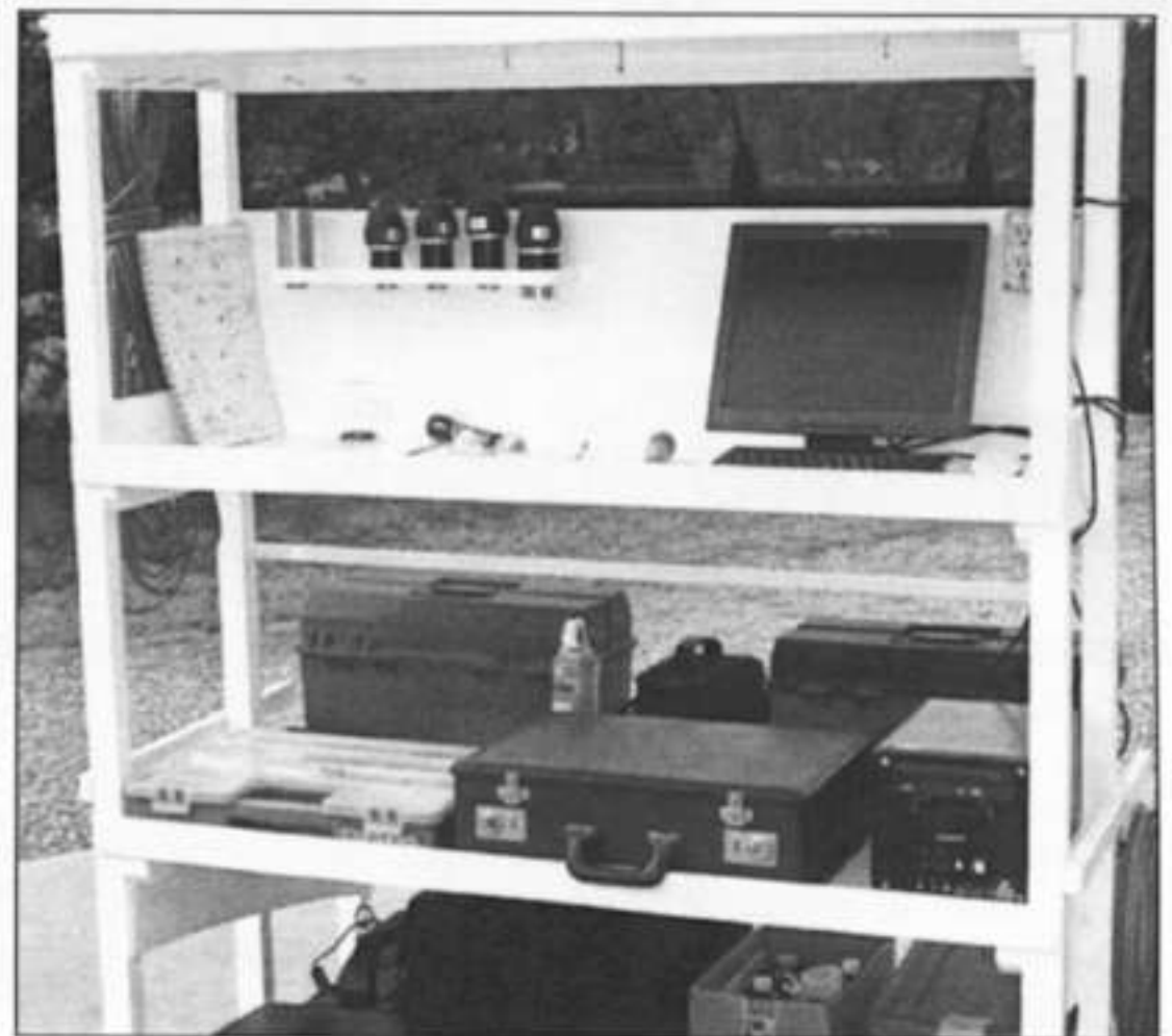
Front view close-up showing eyepiece shelf and equipment layout for observing use. AC receptacle partially hidden by right upright.
